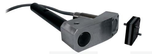
Patented easy to calibrate high-precision measuring gauge featuring a reliable electronic control system.
