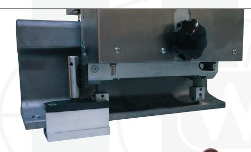
Repeatable measurements possible on the same spot even after grinding the rail track, thanks to a reference bracket that hooks on to the rail track via a handy setscrew. The small and lightweight bracket can be removed and replaced quickly and effortlessly, so multiple measurements can be made along the track.
